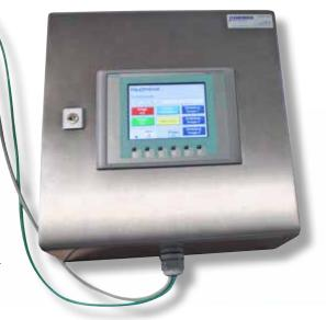
The input of the recipes and dosing batch is done via an elegant display with a keyboard.
